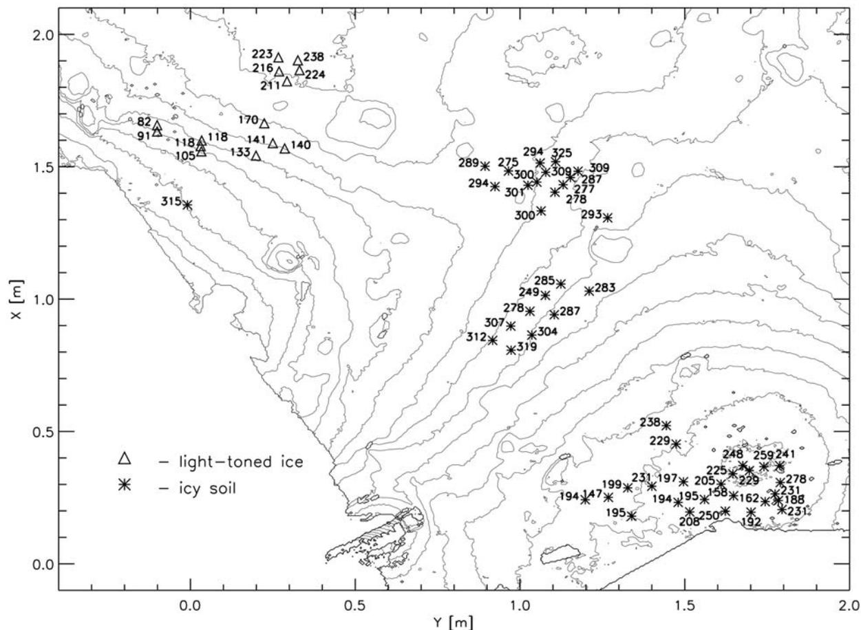
**Figure 9.** Map of the best fitting thermal inertia of the overburden soil assuming a water vapor density of  $3.4 \times 10^{19} \text{ m}^{-3}$ . Thermal inertia values are given in units of  $\text{J m}^{-2} \text{ K}^{-1} \text{ s}^{-1/2}$ . Lower values occur in the soils of the polygon interiors, while higher values occur in the polygon trough regions. The lowest values occur in the scoured region (Figure 6).
