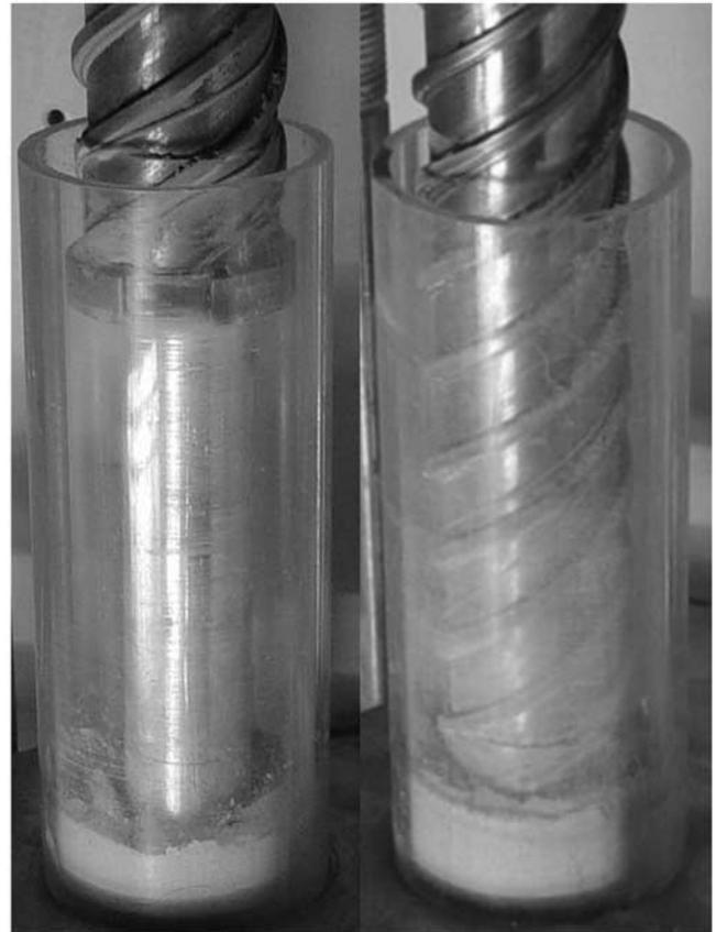
**Figure 2.** Actual experimental arrangement showing the bit with the auger, aluminum core, acrylic tube and rock dust. (left) The drill, metal core, clear tube, and rock powder during a vacuum pumpdown. (right) Prior to gas flushing, the drill was lowered into the tube while rotating.
