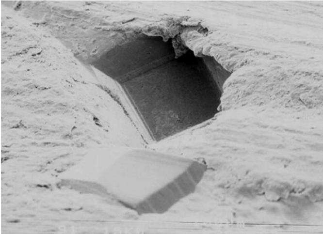
Fig. 2. Diamond pull out due to weak mechanical locking inside the matrix.
